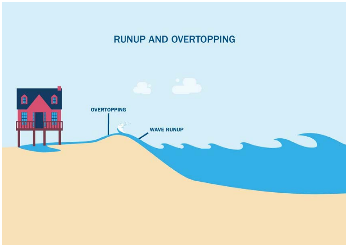
Figure 5b: Wave Overtopping Schematic
